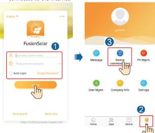
2. Connect to the solar inverter WLAN and log in as **installer** to access the device commissioning screen.
