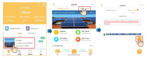
2. Log in to https://intl.fusionsolar.huawei.com to access the WebUI of the FusionSolar Smart PV Management System. On the **Homepage** page, click the plant name to go to the plant page. Select **Plant layout**. Choose — > **Generate with AI**, and create a physical layout as prompted. You can also manually create a physical location layout.
